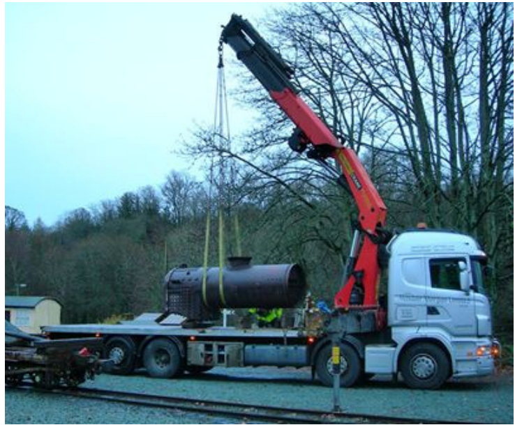
Above 699 boiler loaded for delivery to the SVR
