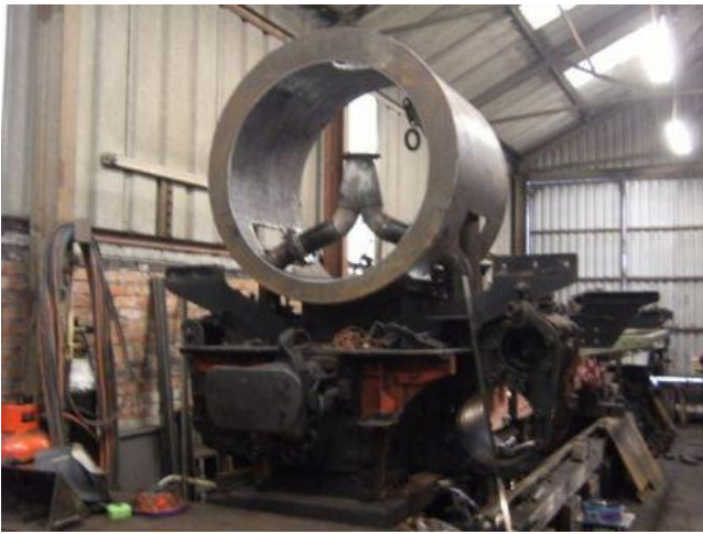
699 stripped right down with a new smokebox being constructed.
